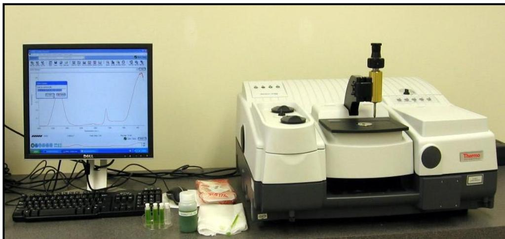
**Figure 3.8:** Nicolet 6700 FTIR-Spectrometer
