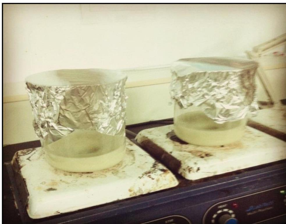
**Figure 3.1:** Methanol and Nanoclay Slurry
