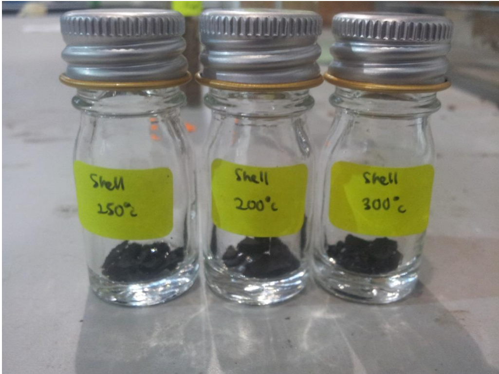
Figure 4-3: Samples of kernel shell after torrefaction
