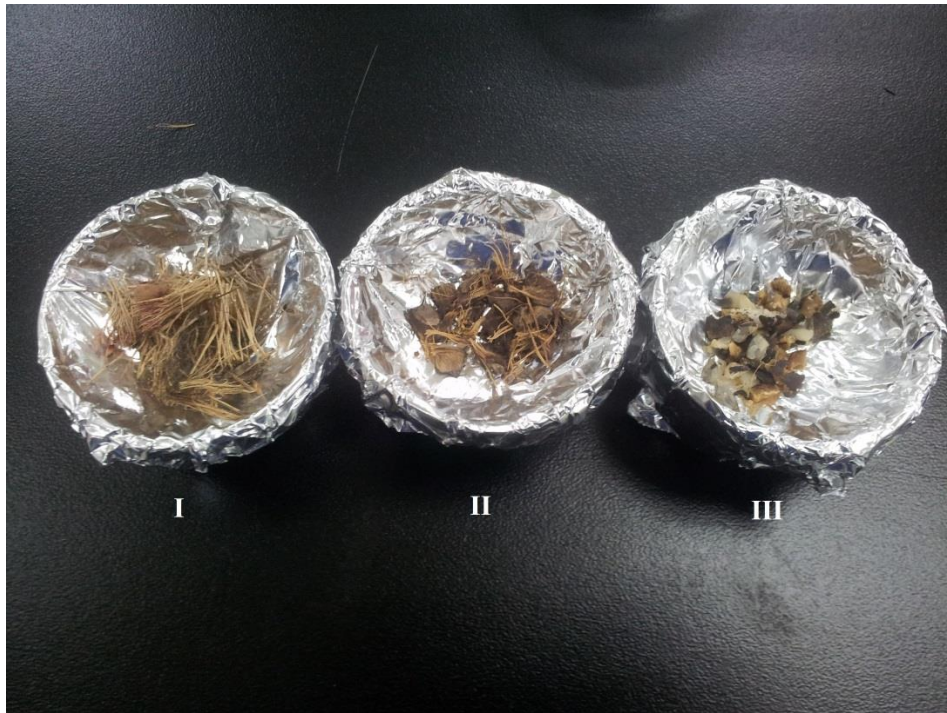
Figure 3-1: Fibrous form of I.) mesocarp fiber, II.) EFB and III.) kernel shell.
