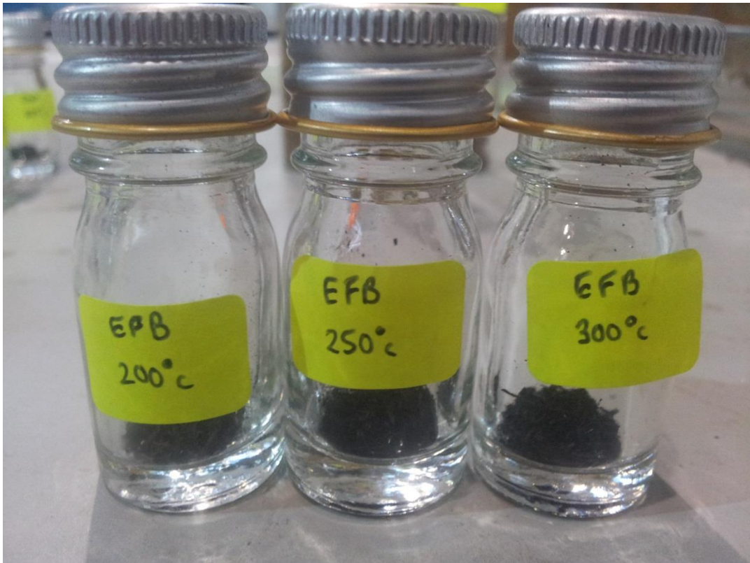
Figure 4-1: Samples of EFB after torrefaction
