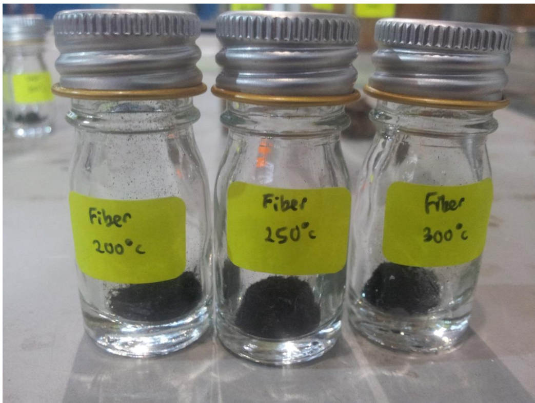
Figure 4-2: Samples of mesocarp fiber after torrefaction
