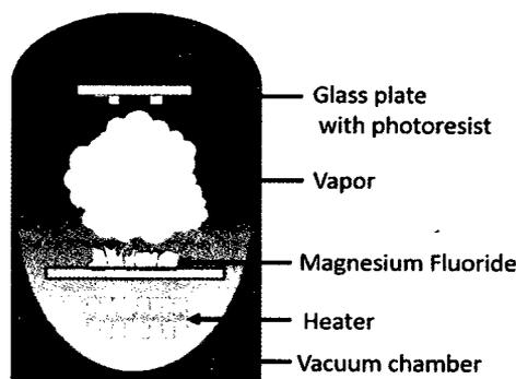
Fig.14 Chemical vapor deposition
