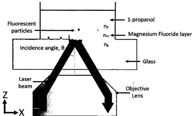
Fig.5 Main concept of Layer TIRF
