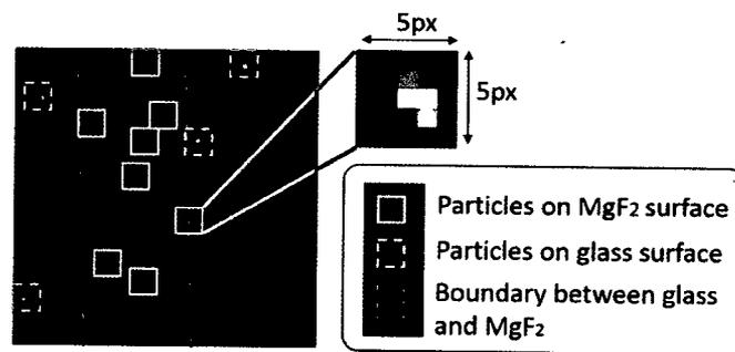
Fig.16 Particle intensity calculation
