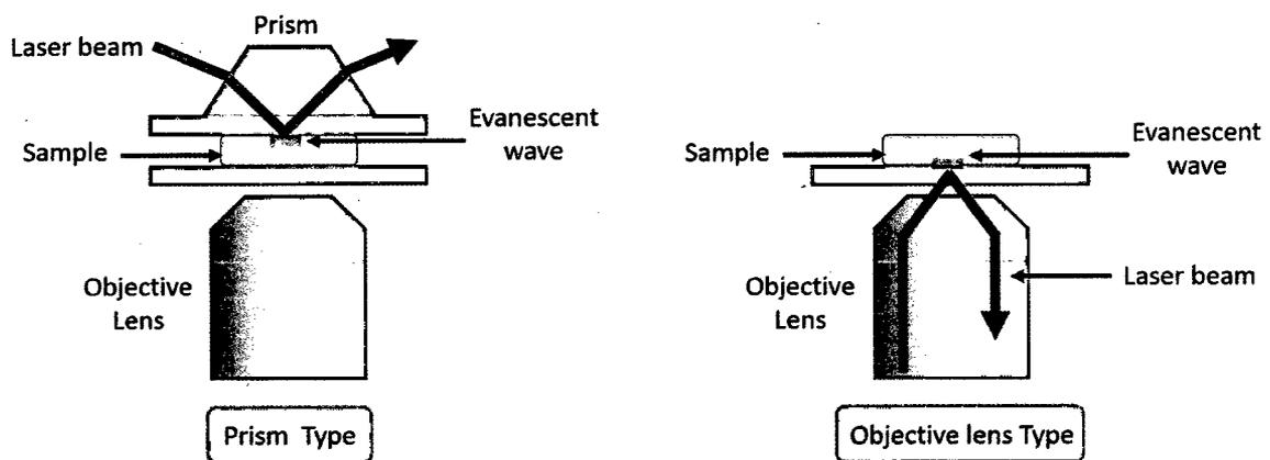
Fig.2 Two different types of TIRF optical system
