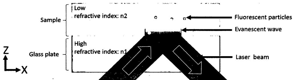
Fig.1 Total Internal Reflection Fluorescence Microscope
