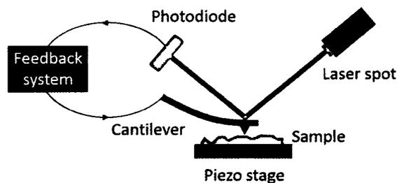
Fig.6 Main principle of atomic force microscopy
