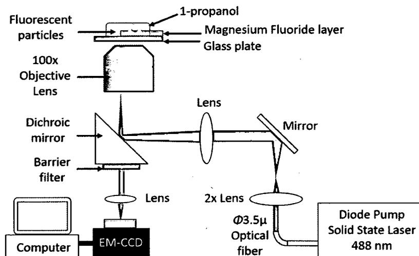
Fig.12 Optical system when using blue laser
