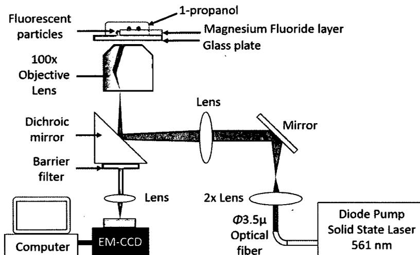
Fig.11 Optical system when using green laser
