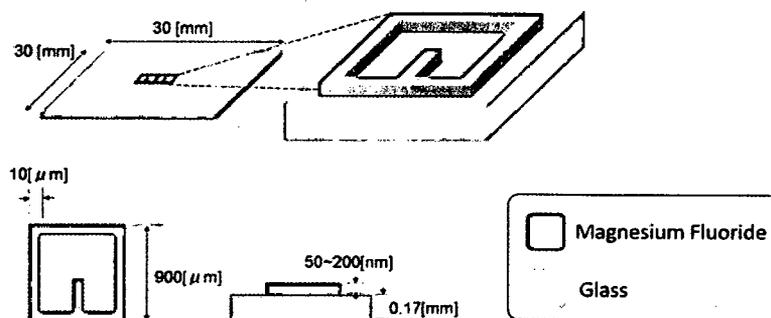
Fig.15 Calibration plate for Layer TIRF
