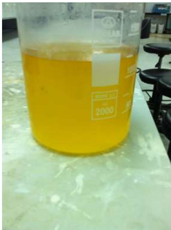
Figure 4: Absolute ethanol which contained dissolved KOH pellets
