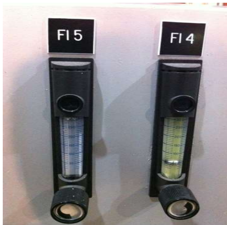
Figure 8: The flow rate of cooking oil (FI 4) and absolute ethanol(FI 5) set at ratio 6:1 which is “50” and “300
