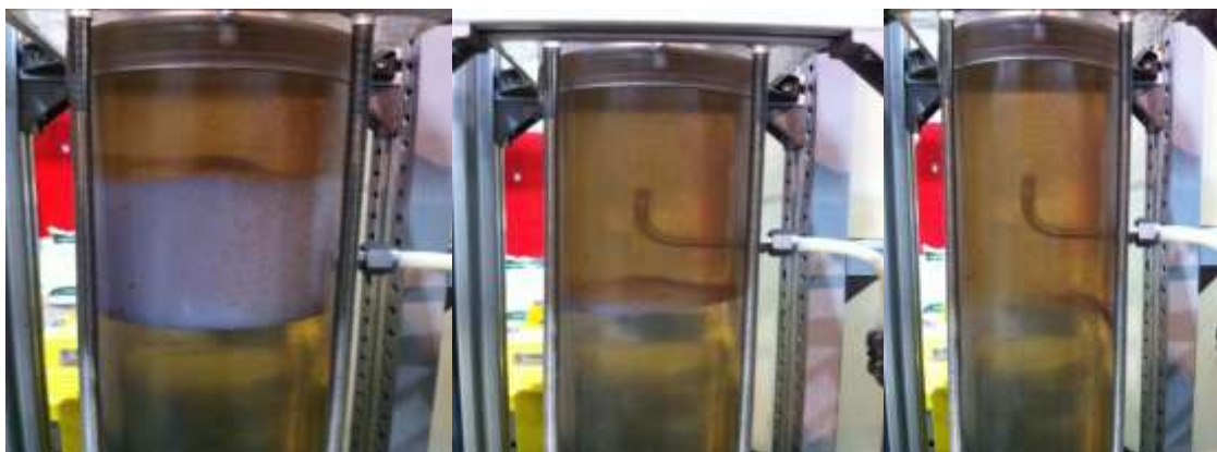
Figure 17: The fatty acid slowly melted from time to time when the heater is turn on.
