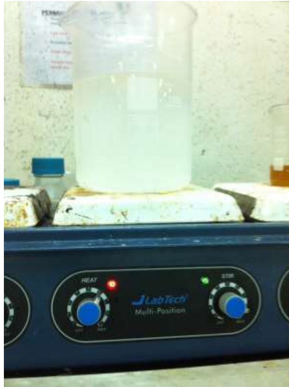
Figure 3: Dissolving KOH pellets using magnetic stirrer
