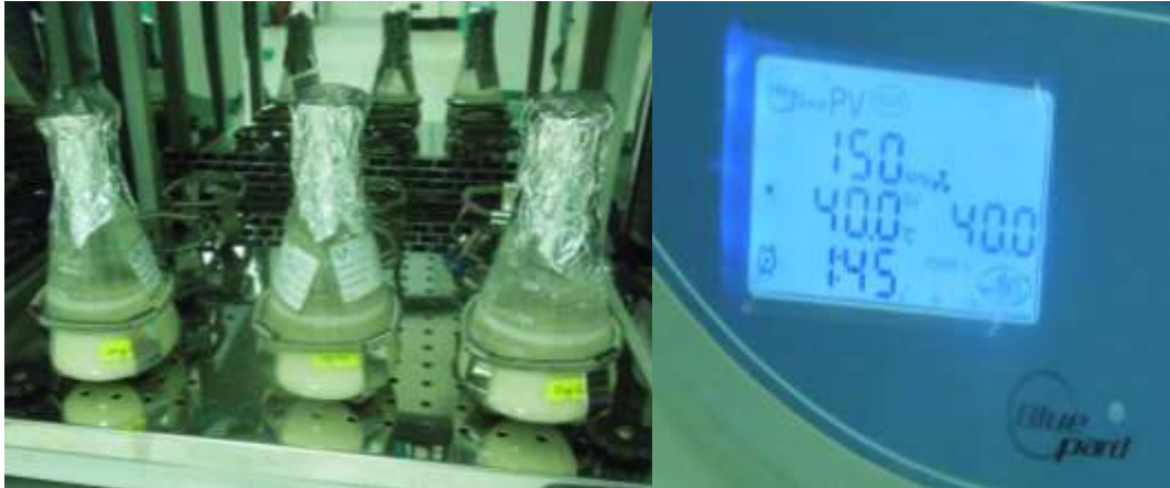
Figure 3-6: Prepared Sample were Kept in Incubator (i.e. at 150 RPM, 40°C and 2 hours)
