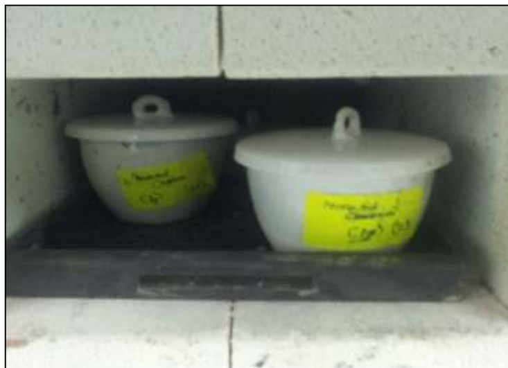
Figure 3-10: Ashing Method (Furnace at 600°C for 24 hours)
