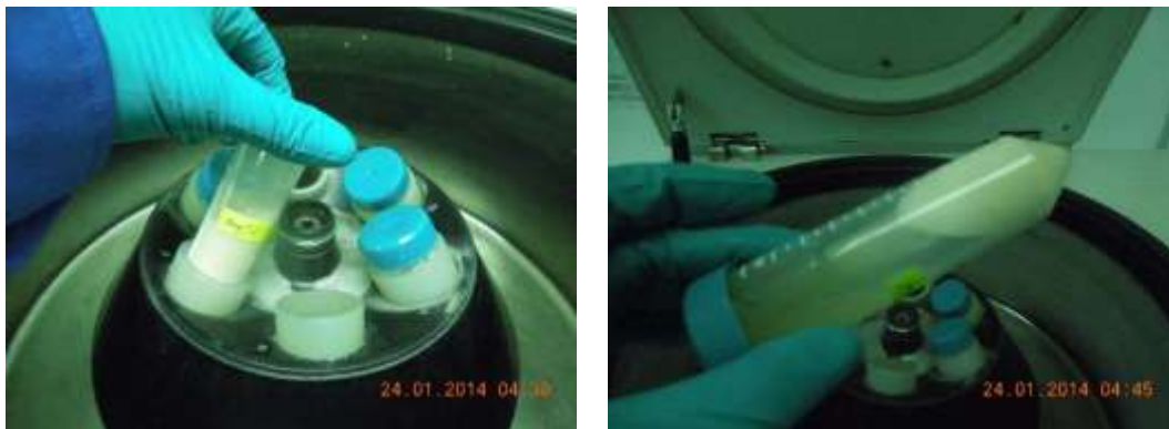
Figure 3-7: Incubated Sample was centrifuged and the Supernatant was removed
