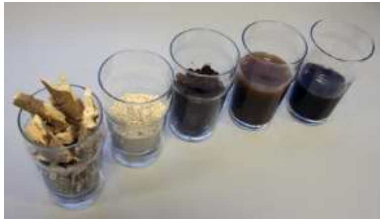
Figure 2-11: How to make biofuel in five easy steps (left-to-right): chipped cassava stalk; milled cassava stalk; after pre-treatment; after enzyme hydrolysis; post-fermentation – the bioethanol “beer”.
