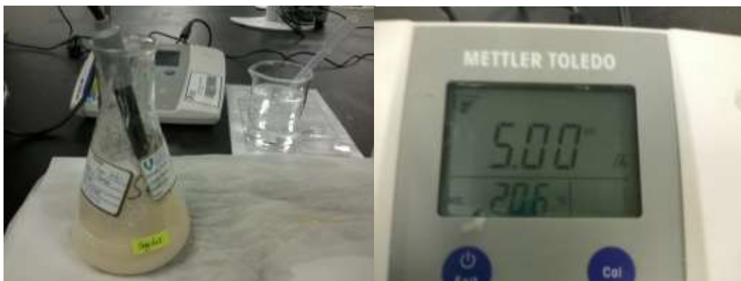
Figure 3-5: The pH value of Solution of Pectinase and Raw Cassava Powder was adjusted using pH meter and either by NaOH or HCL
