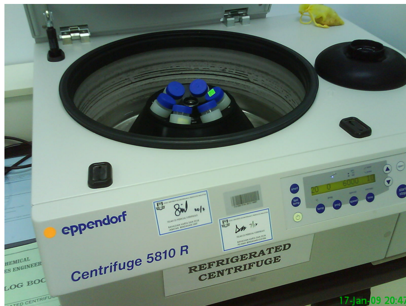
Figure J2 Samples Preparation: Differential Centrifugation of Samples
