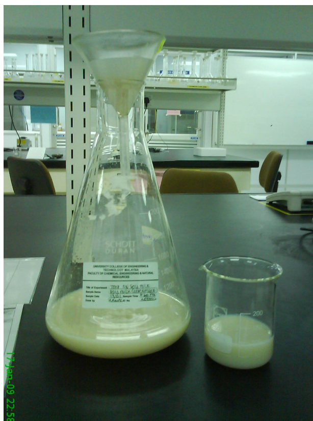
Figure J4 Samples Preparation: Filtration of Samples into Conical Flask
