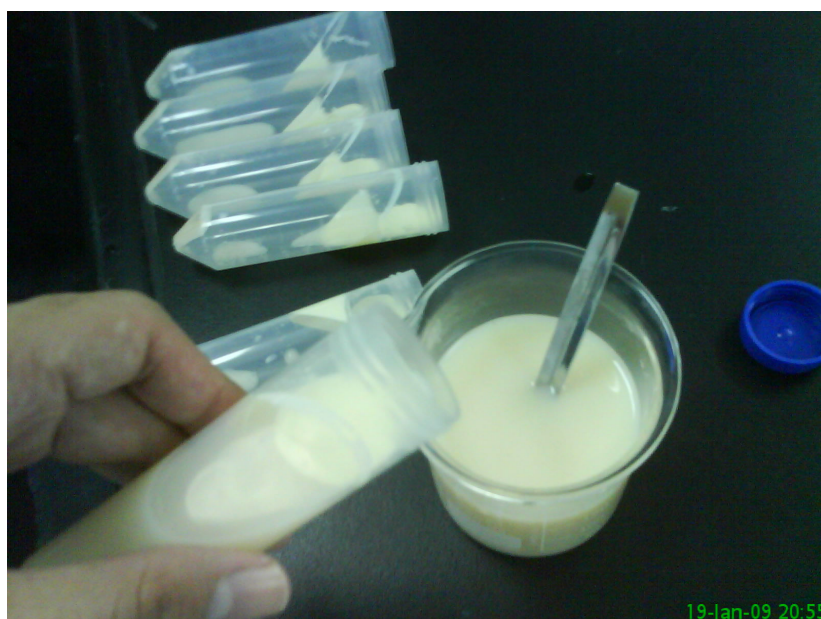
Figure J3 Samples Preparation: Separation of Pellets and Supernatant after Differential Centrifugation Process
