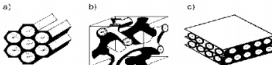
Figure 2-7: Structures of Mesoporous M41S Family: a. MCM-41 (2D hexagonal, space group p6mm ); b. MCM-48 (cubic, space group Ia\bar{3}d ); c. MCM-50 (lamellar, space group p2 ) (Hoffman et al., 2006)
