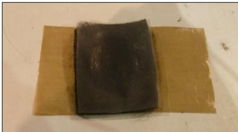
Figure 3-5: Membrane-electrode-assembly (MEA) on Teflon paper
