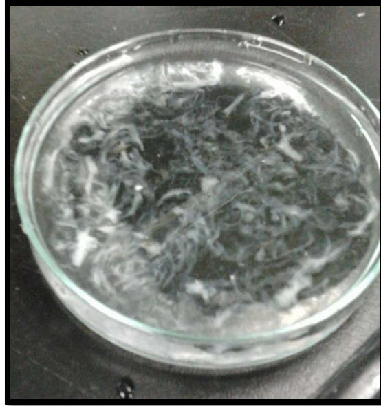
Figure 3-5: The EBN sample with excessive distilled water before filtration
