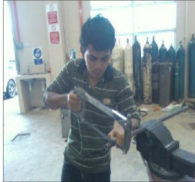
Figure 3.10: Cutting materials by using hand saw
