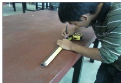
Figure 3.9: Marking the material using steel marker
