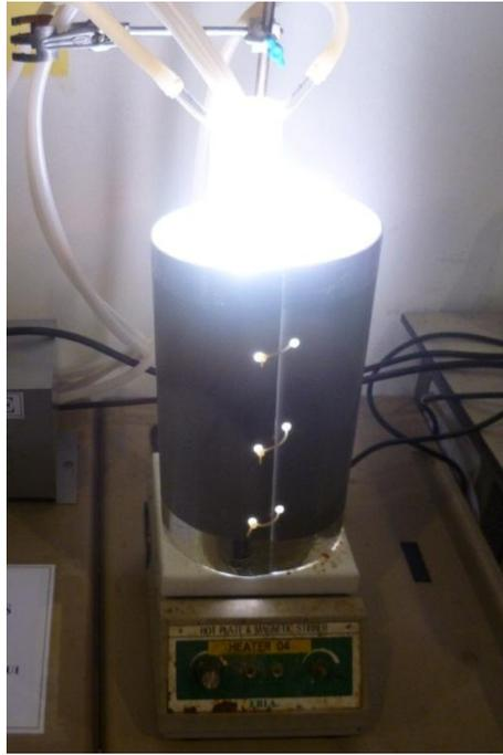
**Figure 3.4** The setup of photoreaction.
