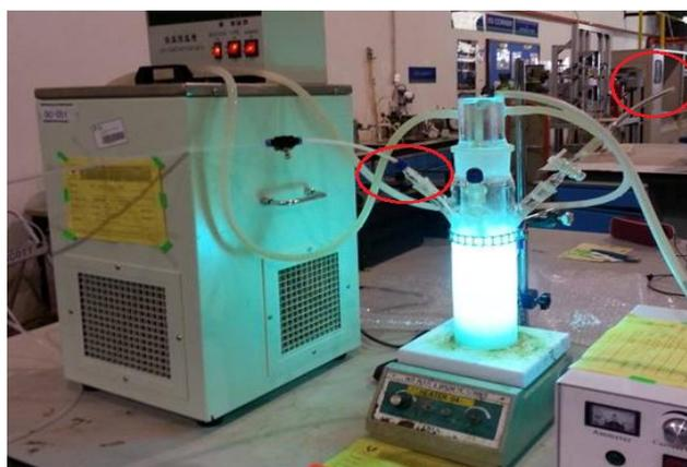
**Figure 4.19** Photoreaction setup to collect gases products.
