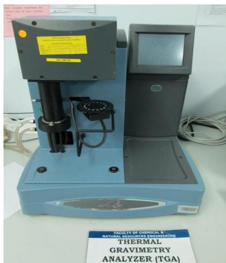
**Figure 3.7:** Thermogravimetric Analysis Q500
