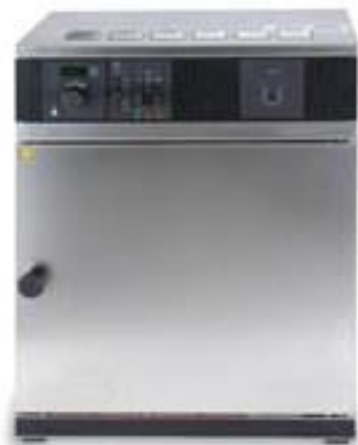
Figure 3.3d: Impregnated activated carbon was heated at 70°C for 6 hours in an oven.
