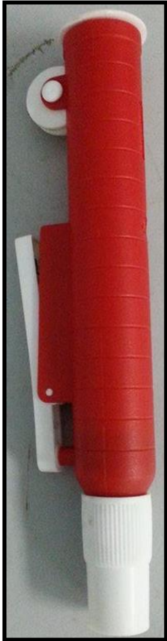
Appendix A.7.3: Hand pump used to pump the biodiesel up to starting point of the viscometer
