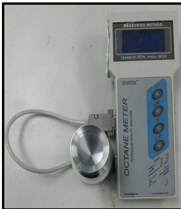
Appendix A.6.1: Shatox SX-100M Portable Octane/Cetane Analyzer
