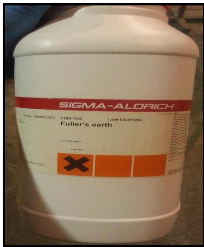
Appendix A.4.6: Fuller's Earth used to bleached crude palm oil
