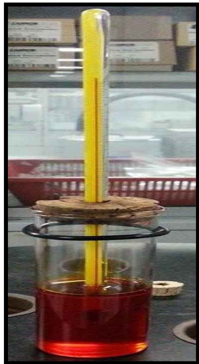
Appendix A.9.2: Test jar containing sample with thermometer
