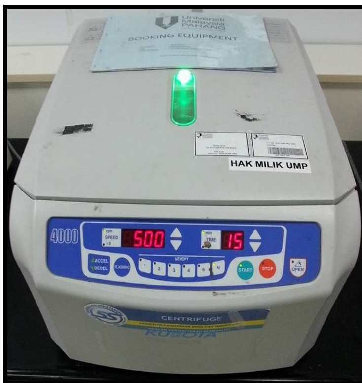
Appendix A.5.9: Centrifuge machine used to separate between florosil and biodiesel
