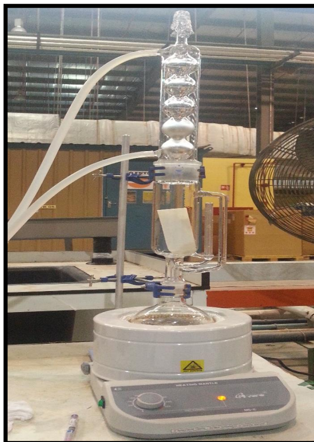
Appendix A.3.4: Oil extraction process using Soxhelt Extractor
