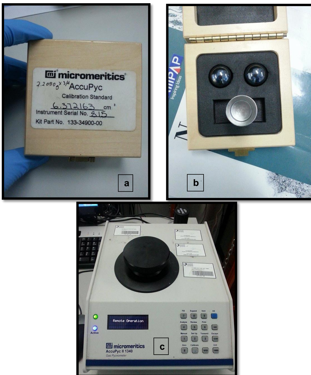
Figure 3.11: a) and b) Chamber used to place the sample c) AccuPyc II 1340 Gas Displacement Density Analyzer (Chamber containing sample will be place inside this machine to be analysed).
