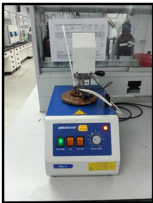
Figure 3.13: Pensky-martens flash point – automatic NPM 440
