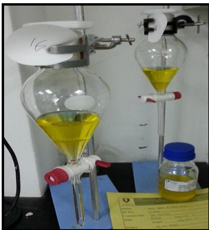
Appendix A.5.4: Settling process ( Moringa oleifera Oil)
