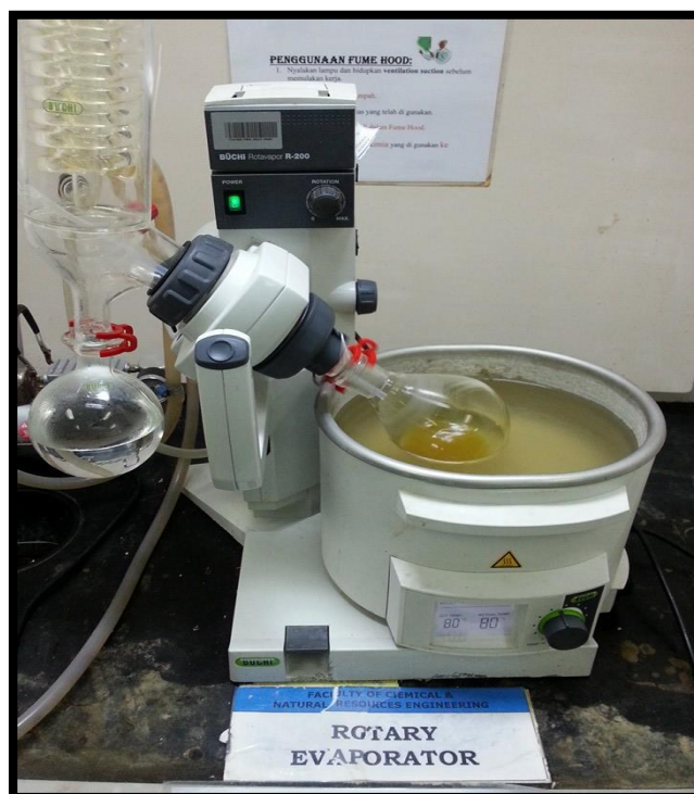
Appendix A.3.6: Separating oil from solvent using rotary evaporator
