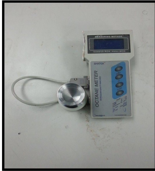
Figure 3.9: Shatox SX-100M Portable Octane/Cetane Analyzer
