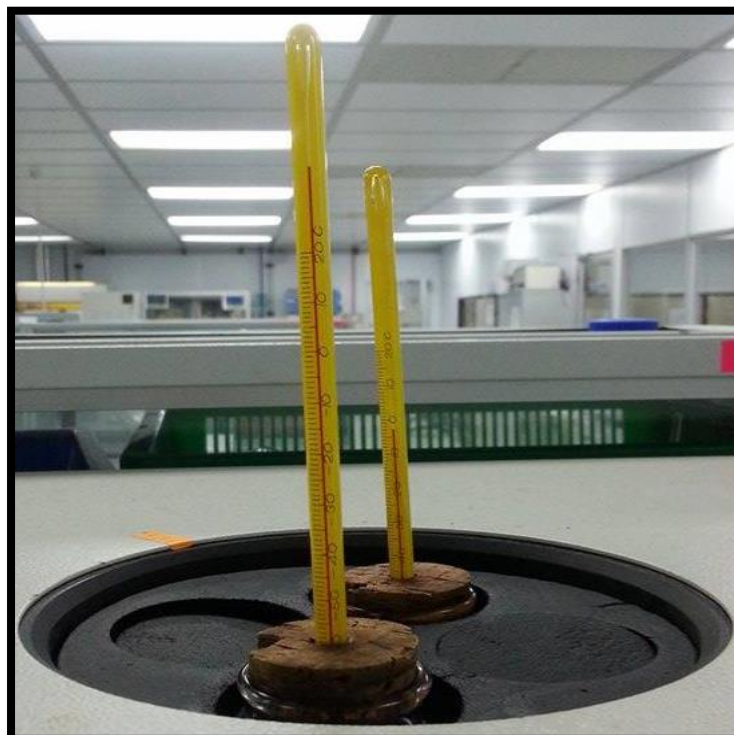
Appendix A.9.4: Test jars with sample inside the K46100 Cloud Point & Pour Point Apparatus
