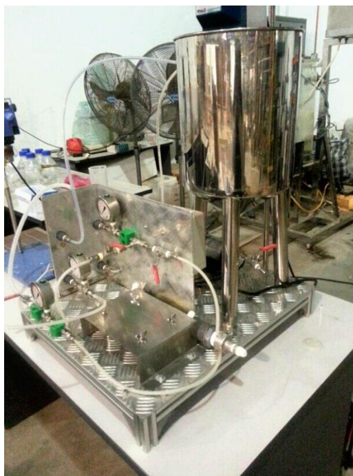
Figure 3.4 Separation equipment use for filtration
