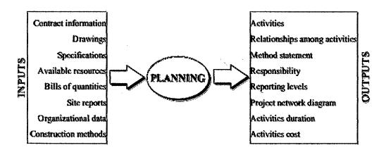
Figure 2.2: Planning inputs and outputs
