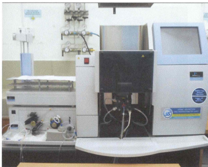
Figure B13: Atomic Absorption Spectrophotometer
