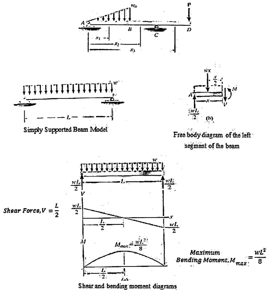
**Figure 2.2:** Shear & Bending Moment diagram based on the Simply Supported Beam as defined in the Mechanics of Materials (Hibbeler R.C, 8<sup>th</sup> ed, p56 – p57)
