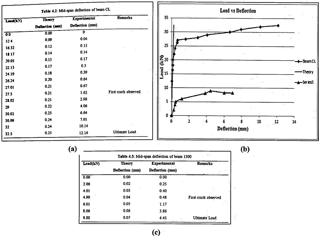
**Figure 2.5:** Load – deflection data and curve from flexural test conducted in laboratory.
