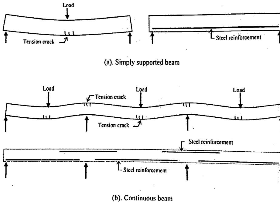
**Figure 2.3:** Behavior of concrete beams in bending (Yassin, 2012)
