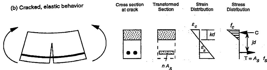
Figure 2.6: Behavior of reinforced concrete beam with increasing bending moment
