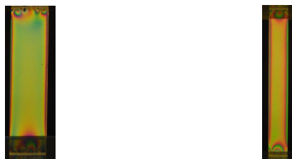
(a) 80mm X 20mm (b) 80mm X 10mm FIGURE 8: Stress distribution by experiment.
