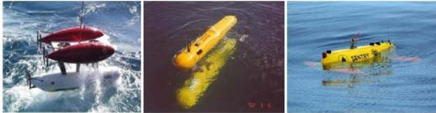
Fig. 5. Non-torpedo shaped AUV.
