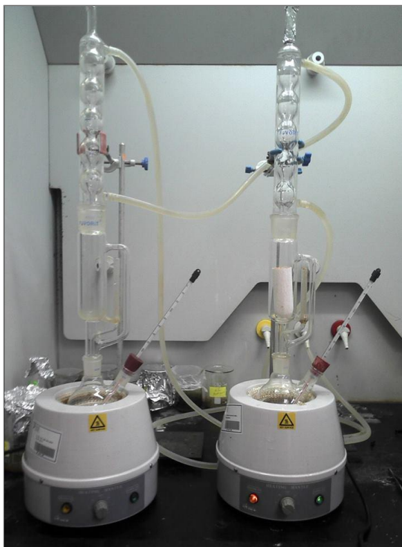
Figure 3.2: Soxhlet extractor used in carotene extraction process
