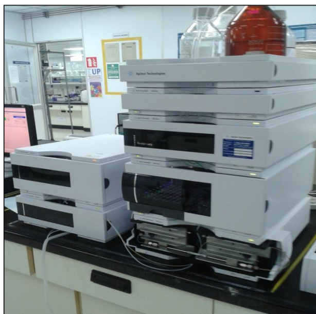
Figure 3.4: High performance liquid chromatography (HPLC) used for analyzing beta-carotene
