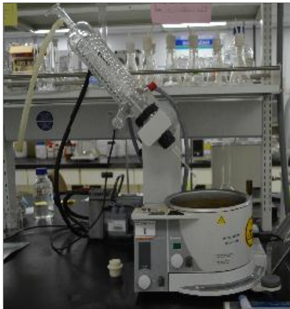
Figure 3.3: Rotary evaporator used for separation process
