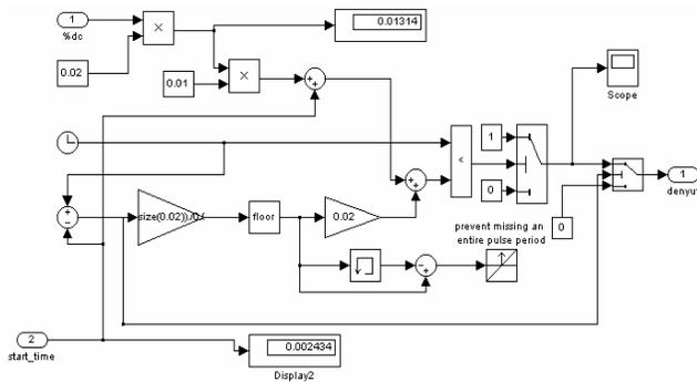
Fig. 3. Subsystem of the Simulink blocks to generate LOGIC 1 and LOGIC 0.
