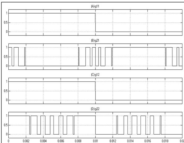
Fig. 9. Gate signals when  $m_i=0.8$  and  $m_f=20$ .
