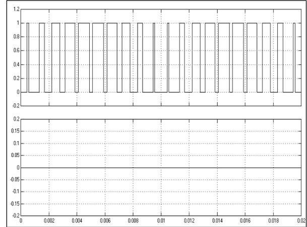
Fig. 5. PWM waveforms of the first (upper) and second (lower) modules of the MSMI for  $mi=0.4$  and  $mf=20$
