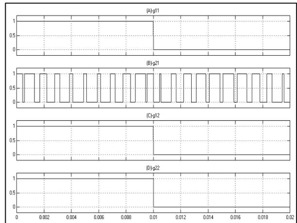
Fig. 6. Gate signals when  $mi=0.4$  and  $mf=20$ .
