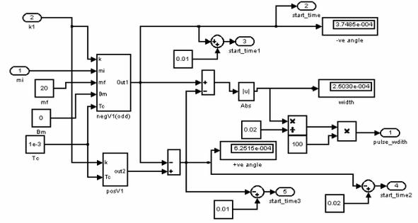
Fig. 2. Subsystem of the Simulink block to generate the timings of LOGIC 1 and LOGIC 0
