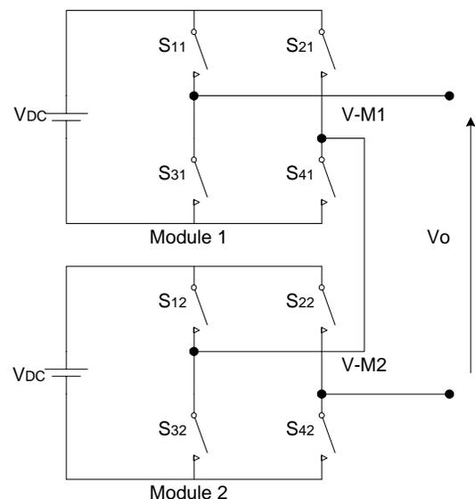
Fig. 1. Single-phase 5-level MSMI configuration
