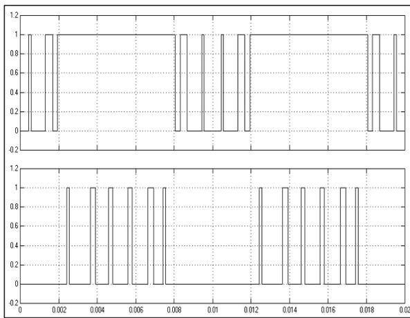
Fig. 8. PWM waveforms of the first (upper) and second (lower) modules of the MSMI for  $m_i=0.8$  and  $m_f=20$
