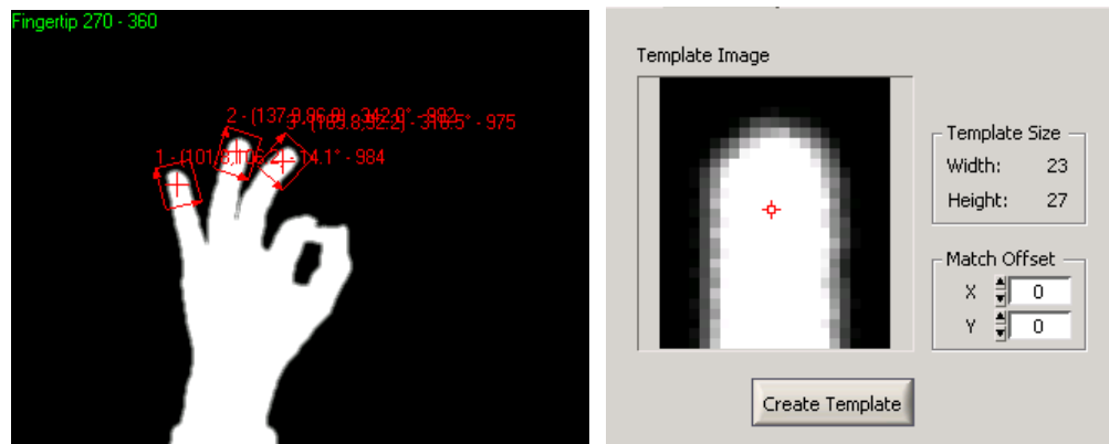
Figure 44: Three fingertips were detected
