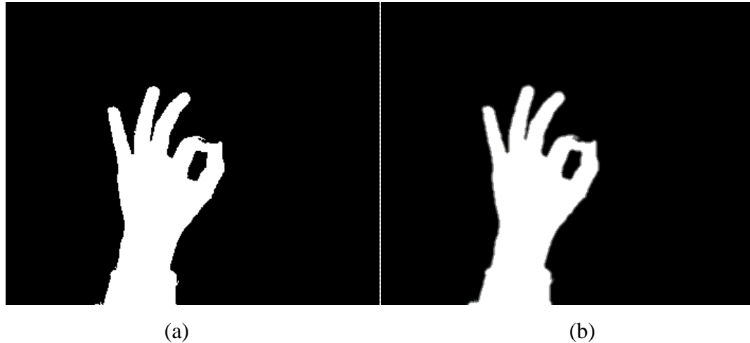
Figure 37: Image Processing Steps (a) Threshold (b) Smoothing
