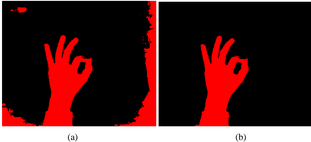
Figure 32: Image Processing Steps (a) Inverse Binary Image (b) Particle Filter
