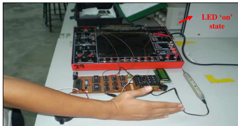
Figure 4.6 Object detected; no signal received by the infrared detector
