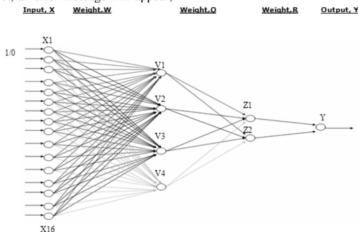
Fig. 2. Neural Network Design for OHMDS
