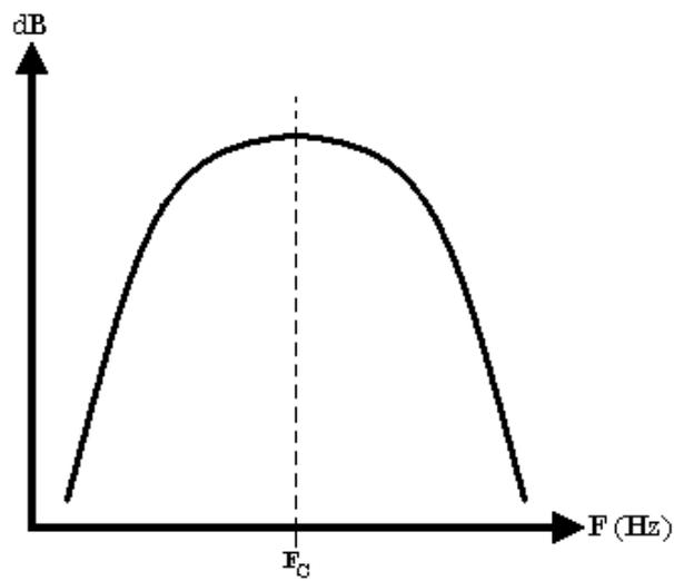
**Figure 2.15 :**  $F_C$  position for bandpass filter
