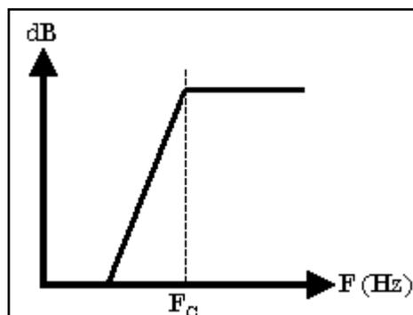
**Figure 2.13 :**  $F_C$  position for high-pass filter
