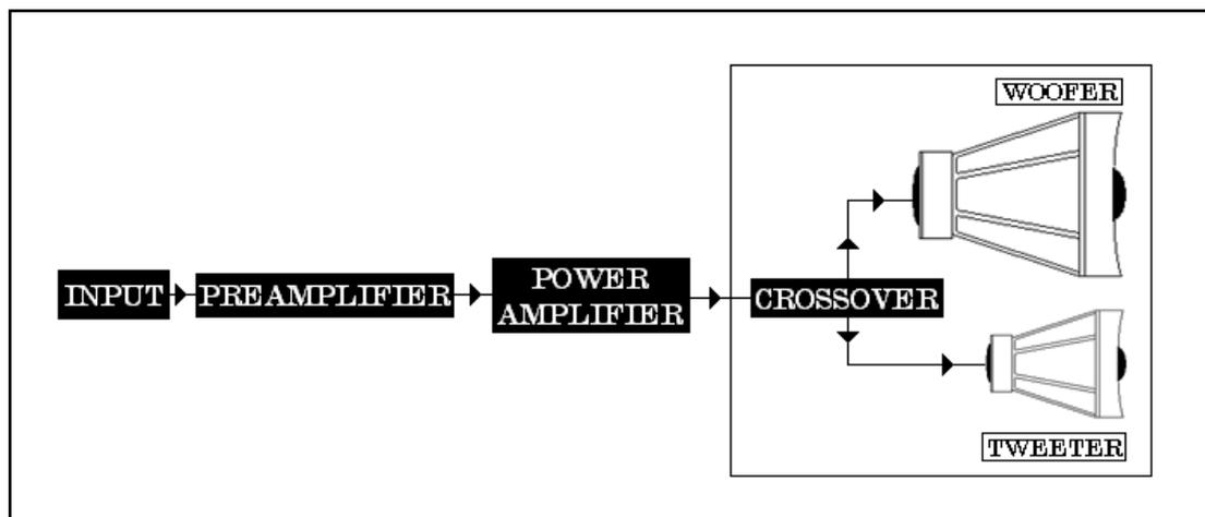
**Figure 2.8 :** Conventional audio system using passive crossover network
