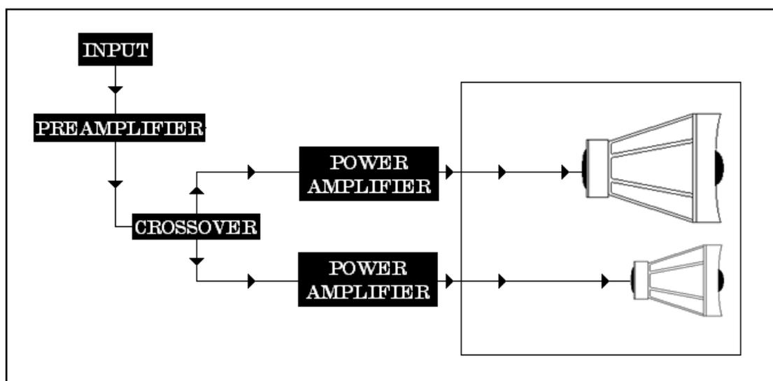
**Figure 2.9** : Conventional audio system using active crossover network
