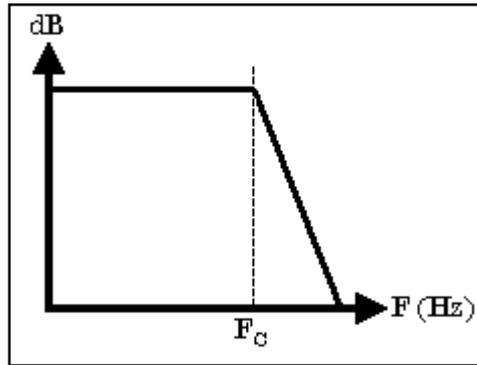
**Figure 2.11 :**  $F_C$  position for low-pass filter
