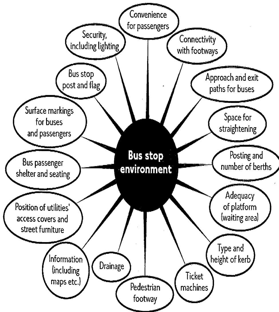
Figure 2.2: Features of the Bus Stop Environment
