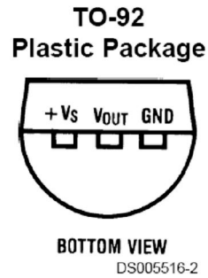
Figure 3.13: Connection Diagram for LM35DZ
