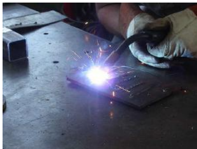
Figure 2.8: Metal Inert Gas (MIG) Welding
