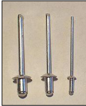
Figure 2.4: Blind Rivet (POP Rivet)
