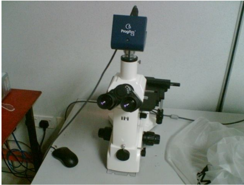
Figure 3.12: Optical Microscope with analyzer ProgRes C3
