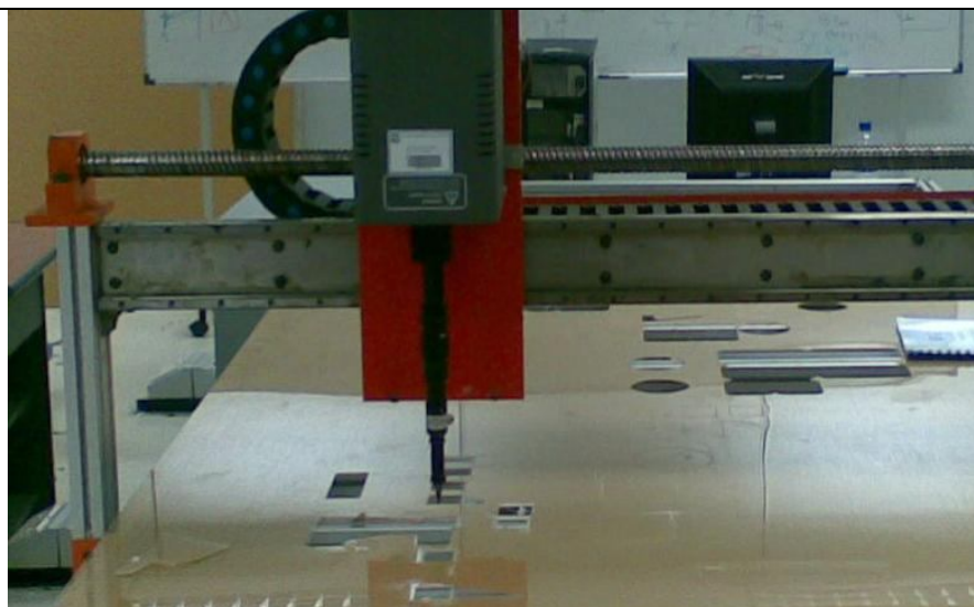
Figure 3.3: ILIOS CO 2 Laser Machine System
