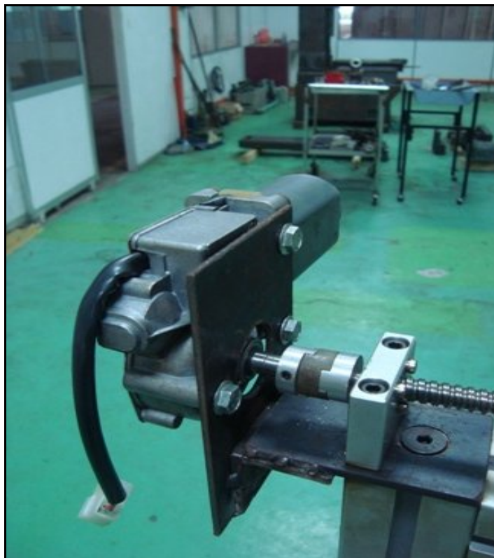
Figure 3.7 : DC motor 1 assembled with ballscrew
