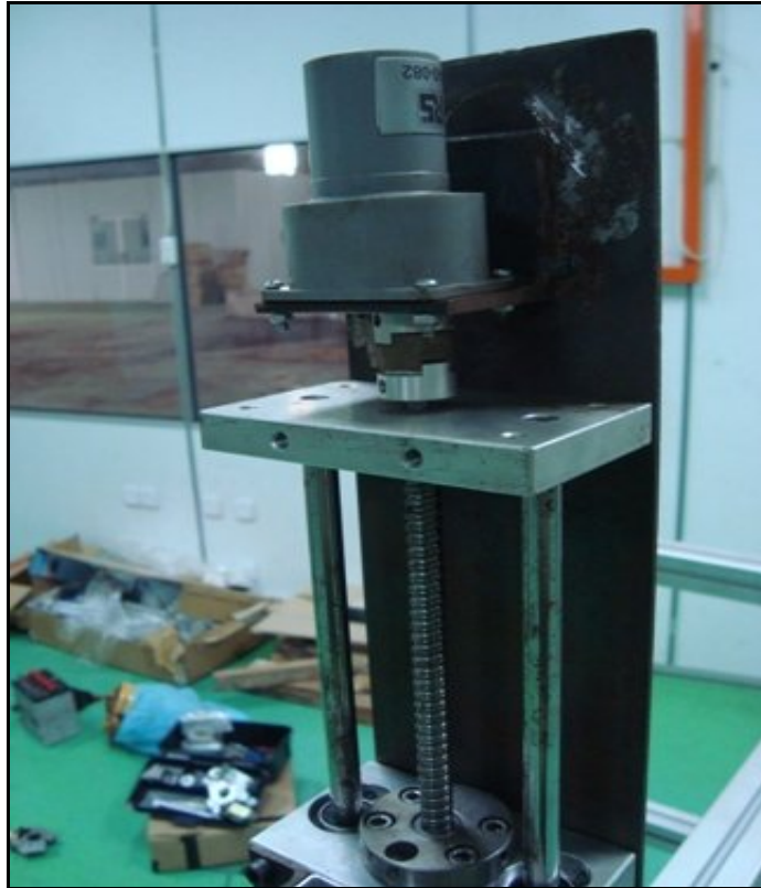
Figure 3.8 : DC motor2 assembled with ballscrew
