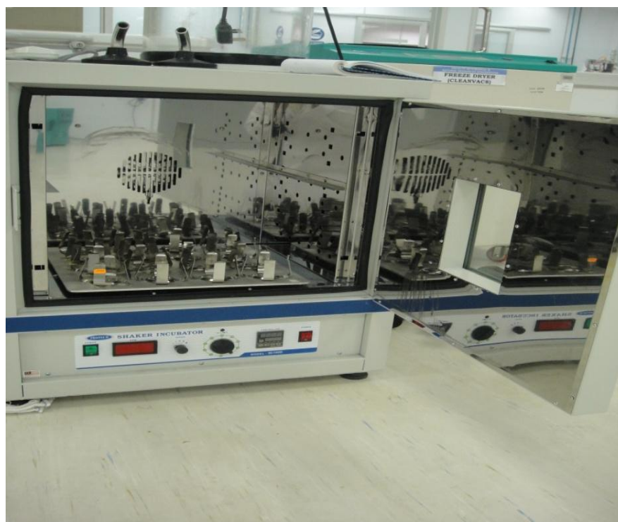
Figure D-5: Hybridization Incubator Shaker model SI-100D,
