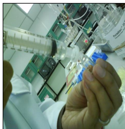
Filtrated sample and filtrated hexane is injected into the vial
