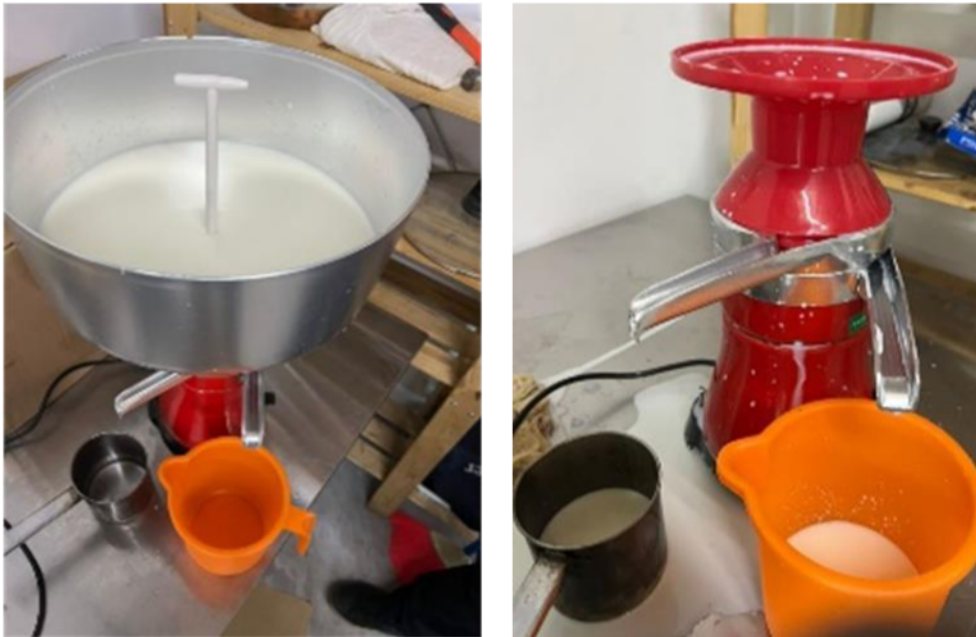
Fig. 3. Diagram of Cream Separator with Leakage of the System due to Excessive Vibration within Parts
